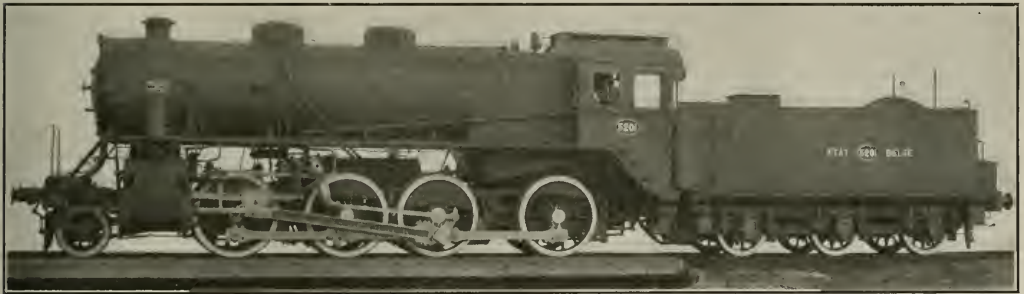
2-8-0 TYPE OF LOCOMOTIVE FOR THE BELGIAN STATE RAILWAYS. American Locomotive Company, Builders.
